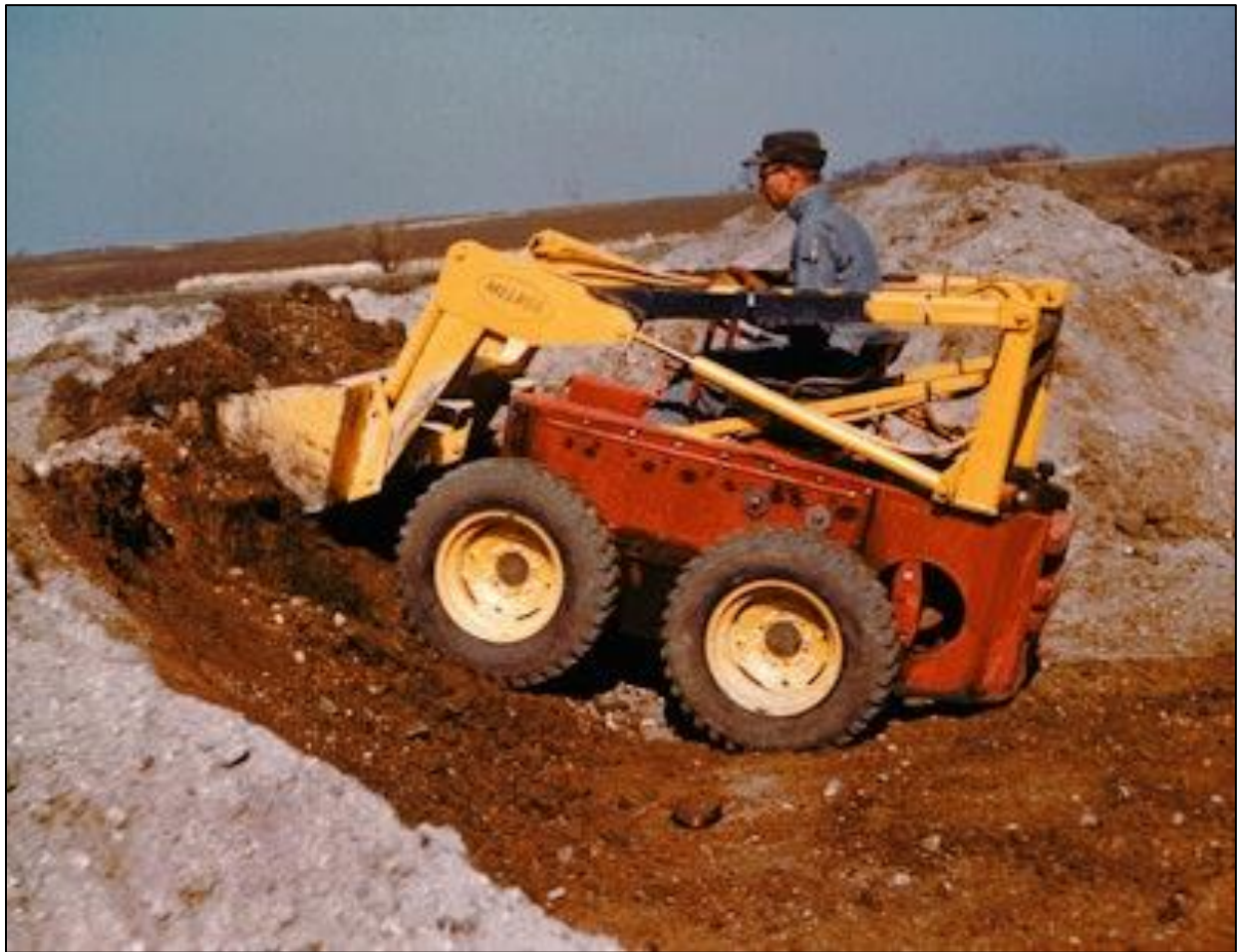
Figure 2: The original Melroe Bobcat (1962), which introduced four-wheel skid-steer to the Kellers’ loaders.
