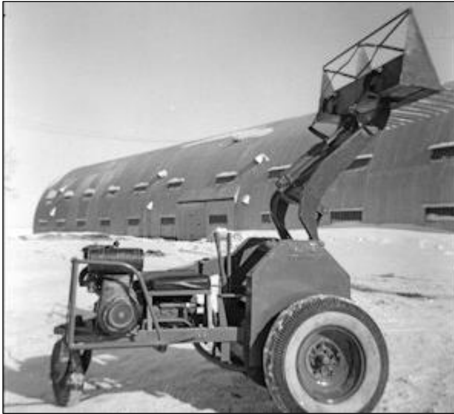
Figure 1: The Keller Self-Propelled Loader, which pivoted on a caster wheel in the rear of the machine.
